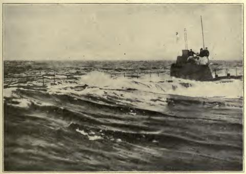
GERMAN SUBMARINE U5, AFTERWARDS CAPTURED BY THE BRITISH IN A STORM This submarine belonged to a class laid down in 1906-07, measured 141 feet 8 inches in length and was armed with two torpedo tubes. When captured, British naval authorities decided that in view of the inhumane conduct of submarine warfare, its authors could not be accorded honorable treatment. Germany immediately declared reprisals, placing British officers in solitary confinement and the original decision was revoked.
